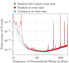
**Figure 1**. Sensitivity of the LIGO detectors at both Hanford and Livingston, shown as noise on the Y axis and gravitational wave frequency on the X axis. The Hanford graph shows noise 4 minutes before the event (grey) which was before the commissioning activity started, and noise during the event (red). Note the much larger noise between about 20 Hertz and 30 Hertz at Hanford during the event. The noise at the Livingston detector is shown in blue. (Adapted from Figure 4 in the <u>paper</u>).
