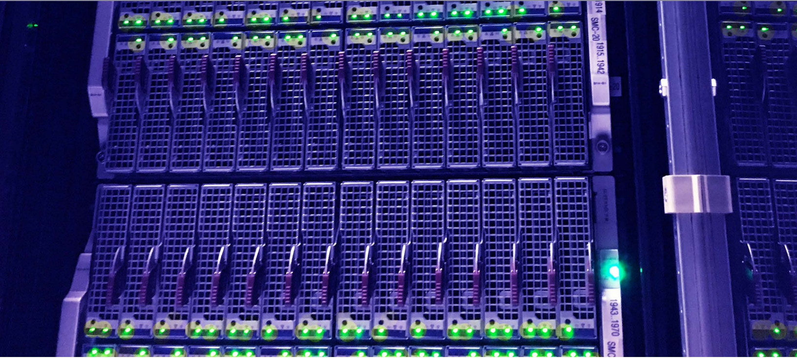
▲ High density Intel Skylake CPU systems installed in the aLIGO datacenter at Caltech to analyze data O2 data.
