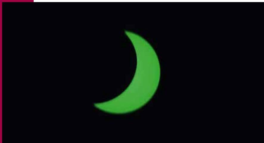
The photo has been taken through a test piece of LIGO black glass mounted on a 80X zoom digital camera. This type of black glass is used for some of the stray light baffles and beam dumps at both observatories. In this case camera magnification was used only to help live streaming on a small digital display. Taken at Caltech.
