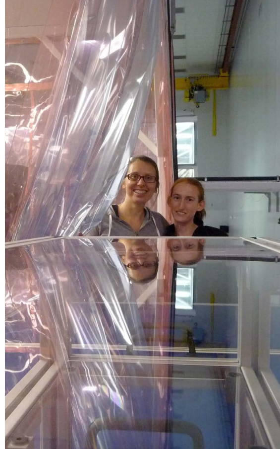
Figure 3: Lisa Barsotti and Sheila Dwyer relax with the squeezer safely installed in its home near the anti-symmetric port. The enclosure around the squeezer prevented dust from getting on the squeezer during the experiment when it could not be inside of a cleanroom because of space constraints.
