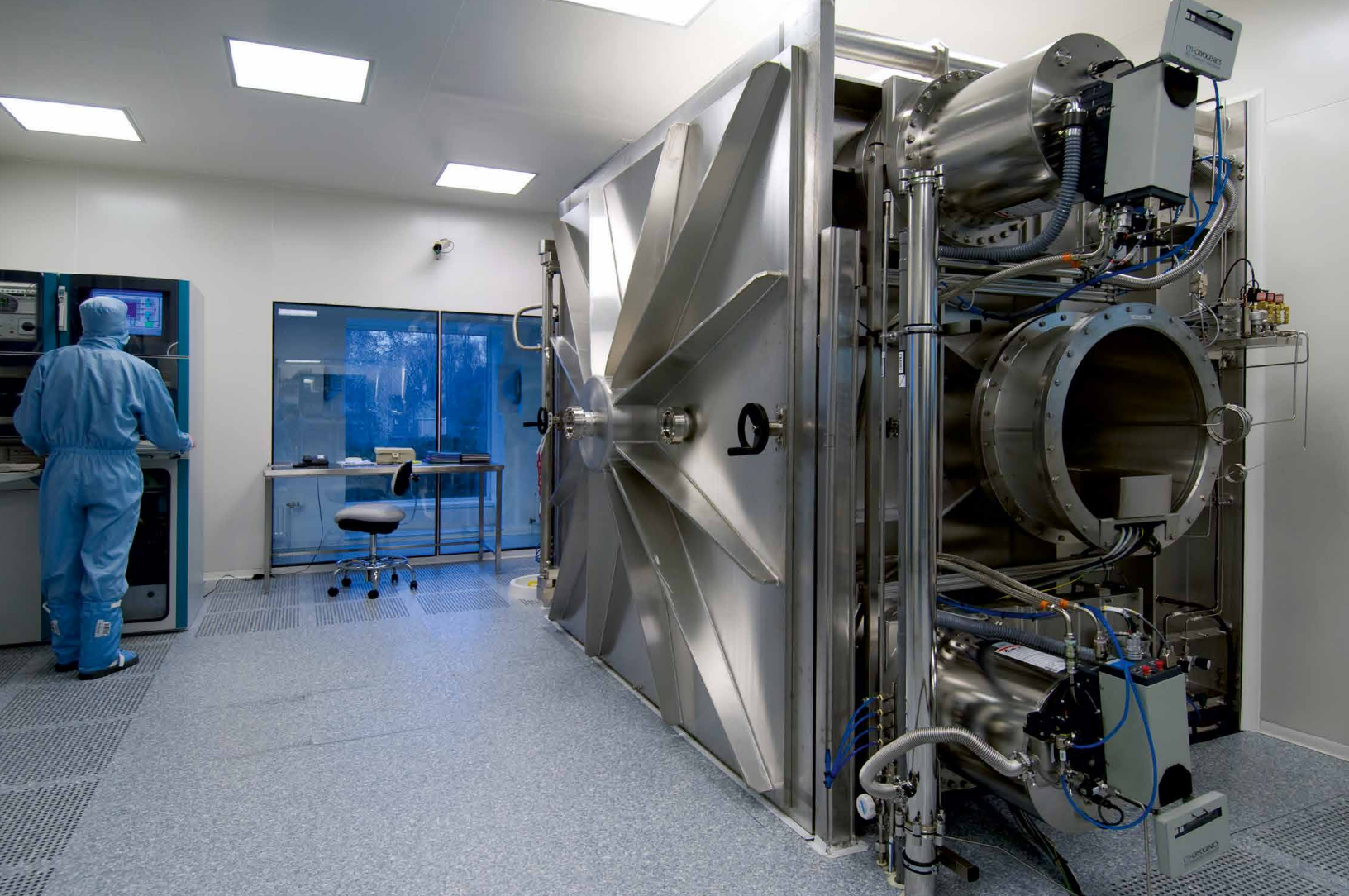
▲ Photo of the largest Ion Beam Sputtering (IBS) coating machine at LMA in which the Advanced LIGO test masses are coated. Thanks to the large coating chamber, two mirrors can be coated at the same time to ensure similar characteristics for both mirrors. The coating machine (as well as the metrology instruments) reside in a class 1 clean room.
