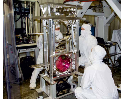
▲ From Left to Right: Gary Traylor, Danny Sellers and Travis Sadecki inspect the ETMX penultimate optic after fiber welding. The welding process involves using a CO2 laser to bond the glass fibers to "ears" on the Test Mass barrel. These welds are then annealed using the same laser. Any imperfections in the weld must be corrected before suspending the 40 kg test mass.
