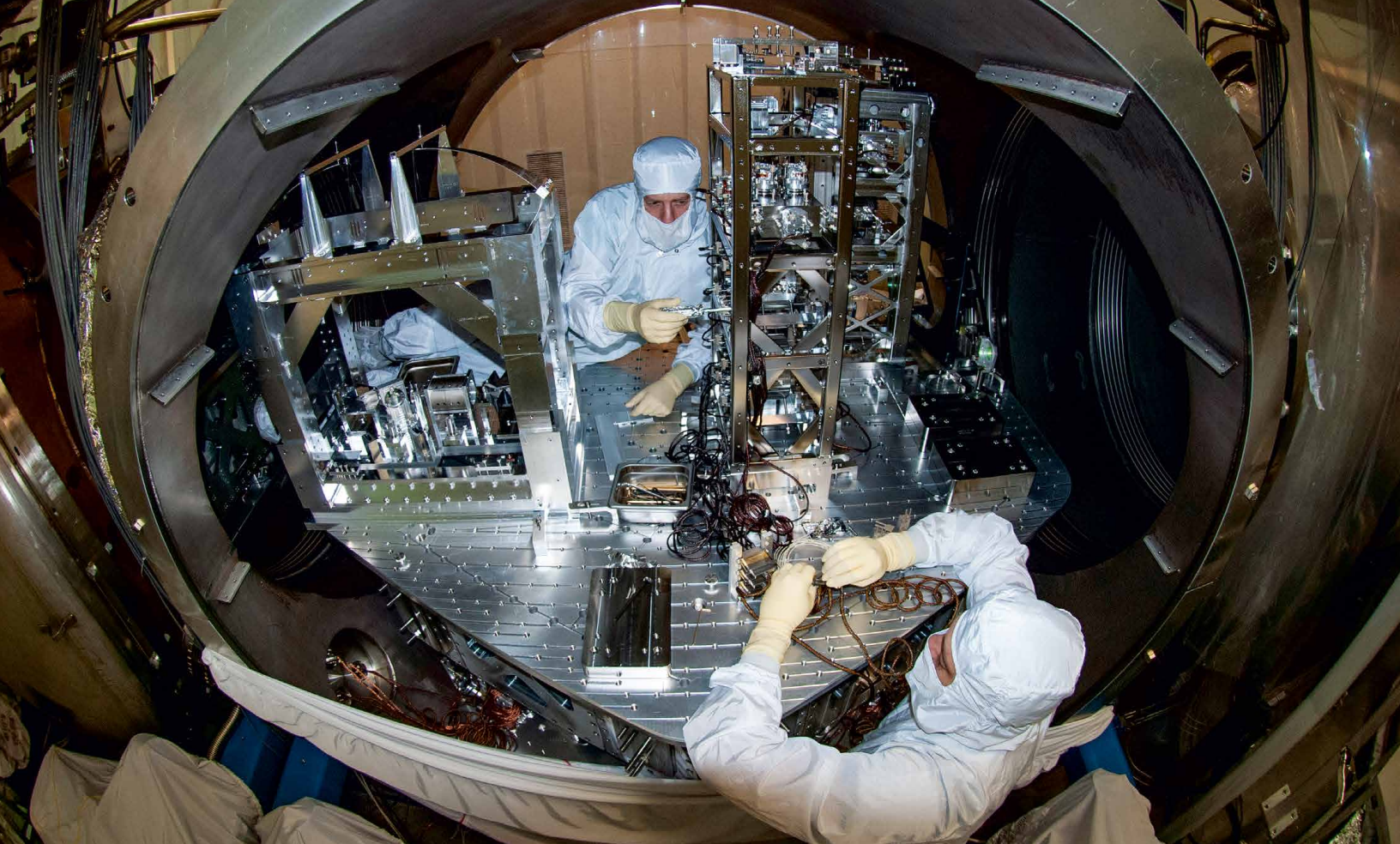
▲ Matthew Heintze (Front) and Danny Sellers (Back) installing suspension cables in HAMS. The Output Faraday Isolator, suspended by wire from two blade springs, is visible on the left. In the foreground on the right is the Signal Recycling Mirror (SRM), and in the background is the SR3 suspension.
