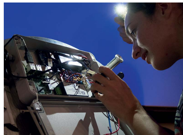
Members of the Birmingham outreach team during the first day of installation. Top and Middle: fitting the leg and feeding cabling from the Michelson and Pi to the Thinktank's main system; Bottom: a snug fit inside the control box, which houses everything used to control the exhibit from the laser power supply to the Raspberry Pi and Arduino.
