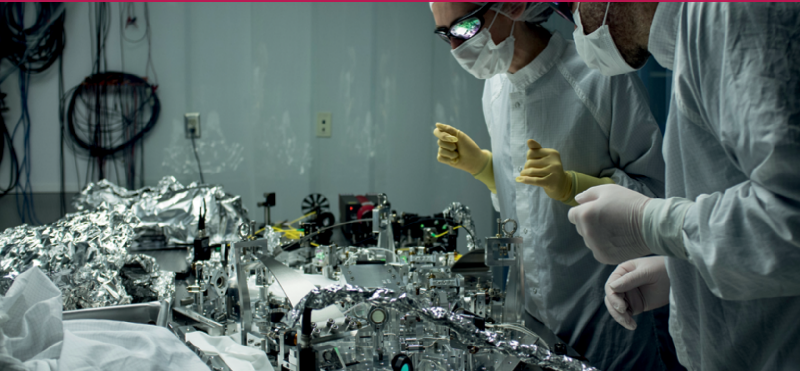
▲ Installing the squeezer at Hanford.
