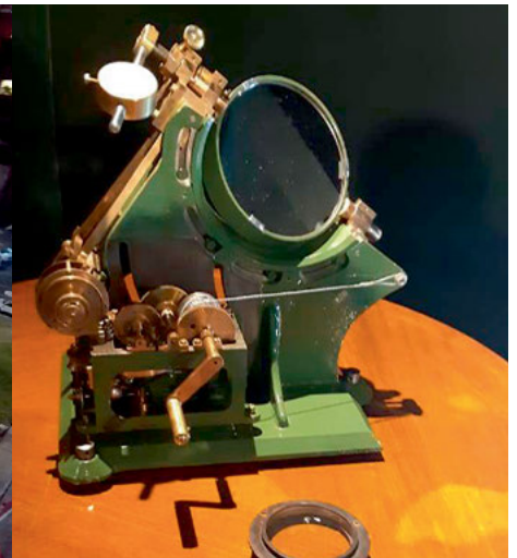
Left image: Bird's eye view of the celebrations in Sobral. Right image: The 4-inch lens and 8-inch coelostat of the telescope which recorded the eclipse images. They were presented to the public of Sobral having been lost and found in the Dunsink Observatory storage after 70 years.
