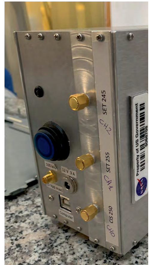
TRL4 prototype CMD, developed by the Precision Space Systems Lab at the University of Florida, delivered to the University of Trento for GRS subsystem-level testing.
