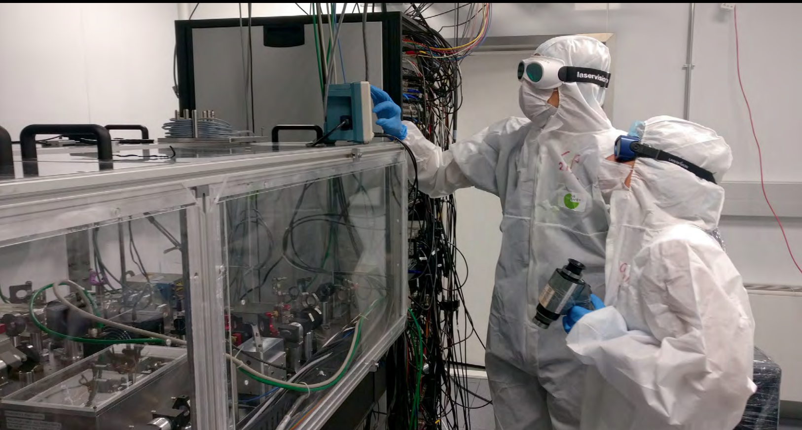
Scattered light noise hunting in the Advanced Virgo Laser laboratory. The Laser bench is visible on the left.
