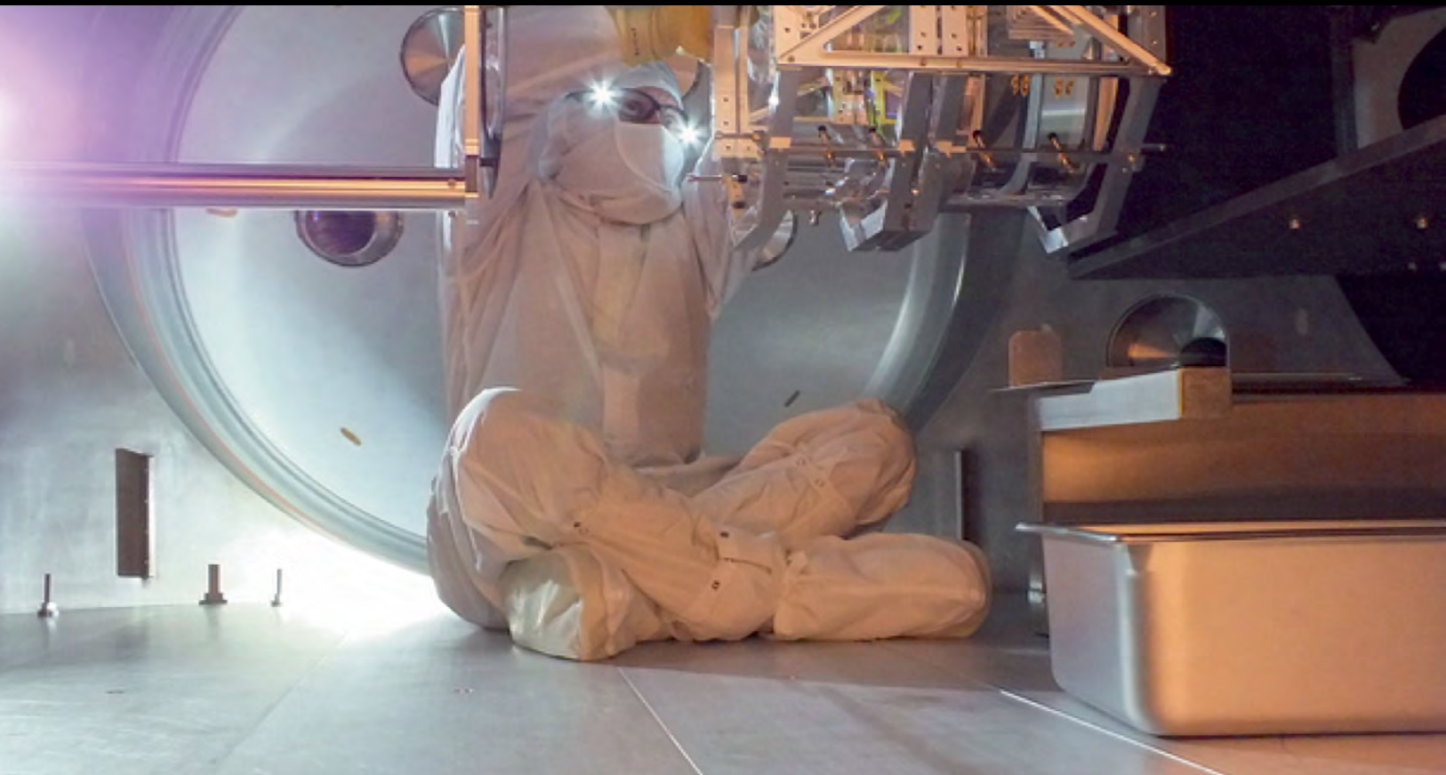
▲ Unlocking one of the end test-masses (mirrors) after cleaning at Livingston.
