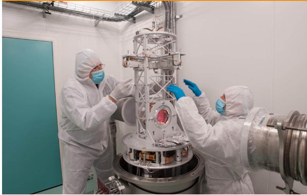
▲ Installation of the input mirror suspension, composed by two pendulum stages sitting on a pre-isolator constituted by an inverted pendulum.
