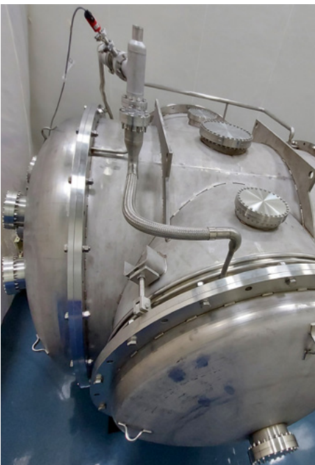
▲ Factory testing of the HAM Chamber.
