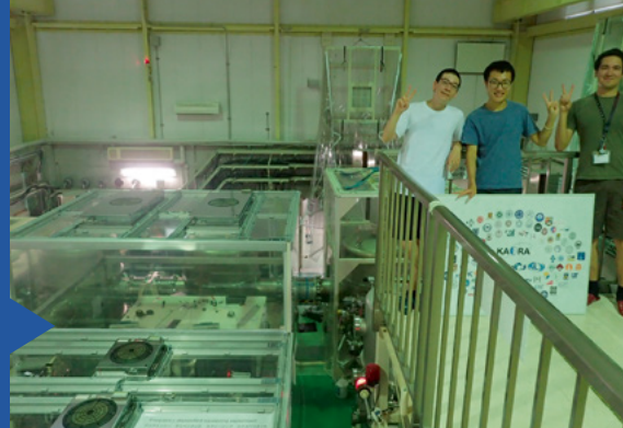
A 300m filter cavity prototype located in NAOJ, Japan, using the infrastructure of TAMA300. An in-air squeezer produces frequency independent squeezing and goes to an in-vacuum 300m filter cavity to become frequency dependent squeezing. The squeezer is in the cleanroom on the lower left side of this photo. The door for the filter cavity is in the middle of this photo. (Marc Eisenmann, Yuhang Zhao, Michael Page).
