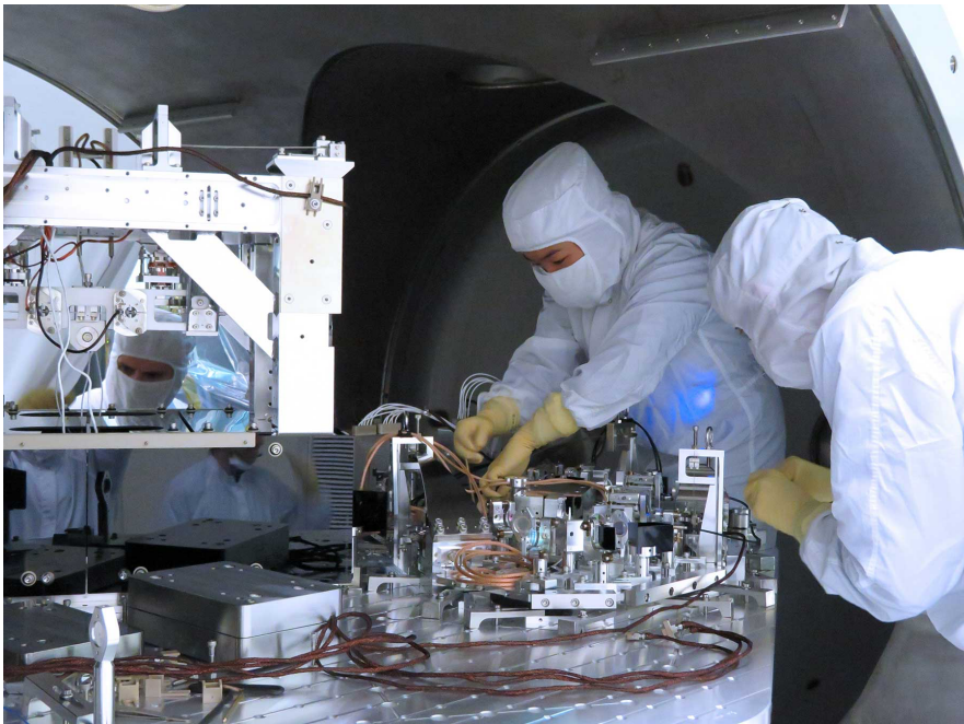
LIGO team members install in-vacuum equipment that is part of the squeezed-light upgrade. [Image credit: LIGO/Caltech/MIT/Matt Heintze]
