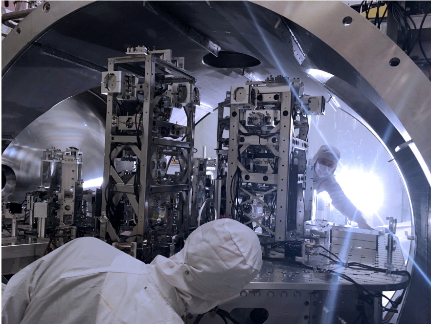
Detector engineers Hugh Radkins (foreground) and Betsy Weaver (background), are pictured here inside the vacuum system of the detector at LIGO Hanford Observatory, beginning the hardware upgrades necessary for Advanced LIGO's third observing run. [Image credit: LIGO/Caltech/MIT/Jeff Kissel]
