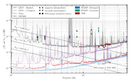
**Figure 1**: Noise spectrum of the gravitational-wave detectors (solid lines) and the amplitude of gravitational waves required to detect 50% of simulated signals (triangles and squares). The dashed black line corresponds to the physical limit in the parameter space, above which more energy is emitted than in the measured total mass of the binary. Open squares represent realistic model predictions for <1 second long signals.
