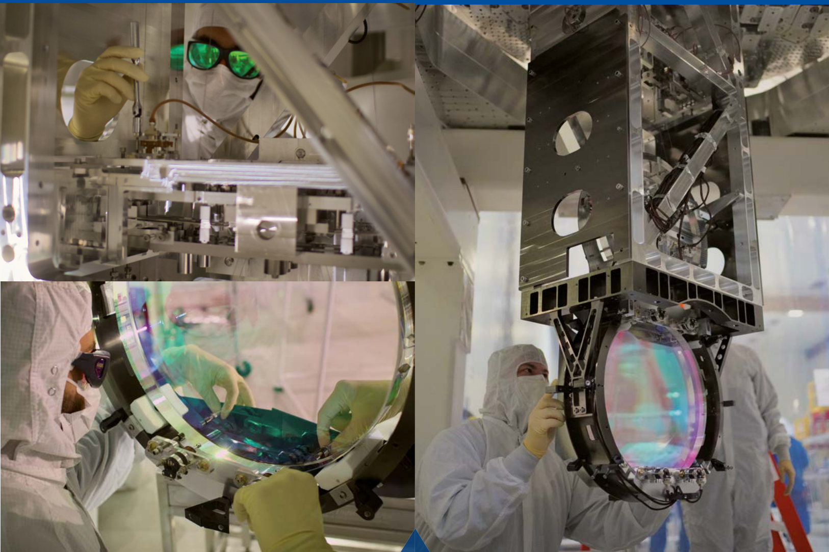
Top left: Tom adjusting the alignment of a QOSEM on the Bigger Beamsplitter Suspension. Out of picture Oli is checking the readings from the sensor, helping guide it into position. Bottom left: Ibrahim and Tom placing rubber earthquake stops on the beamsplitter, desuspending the optic and preventing it from moving during its craning into the vacuum chamber. Right: TJ installing a protective metal cover in front of the beamsplitter optic, to prevent any accidental knocks or scratches while working on the suspension system above.
